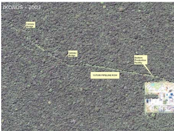
Fig. 8 – High-resolution IKONOS imagery (1 meter pixel) showing narrow pipeline ROW and canopy bridges near the EPF.
